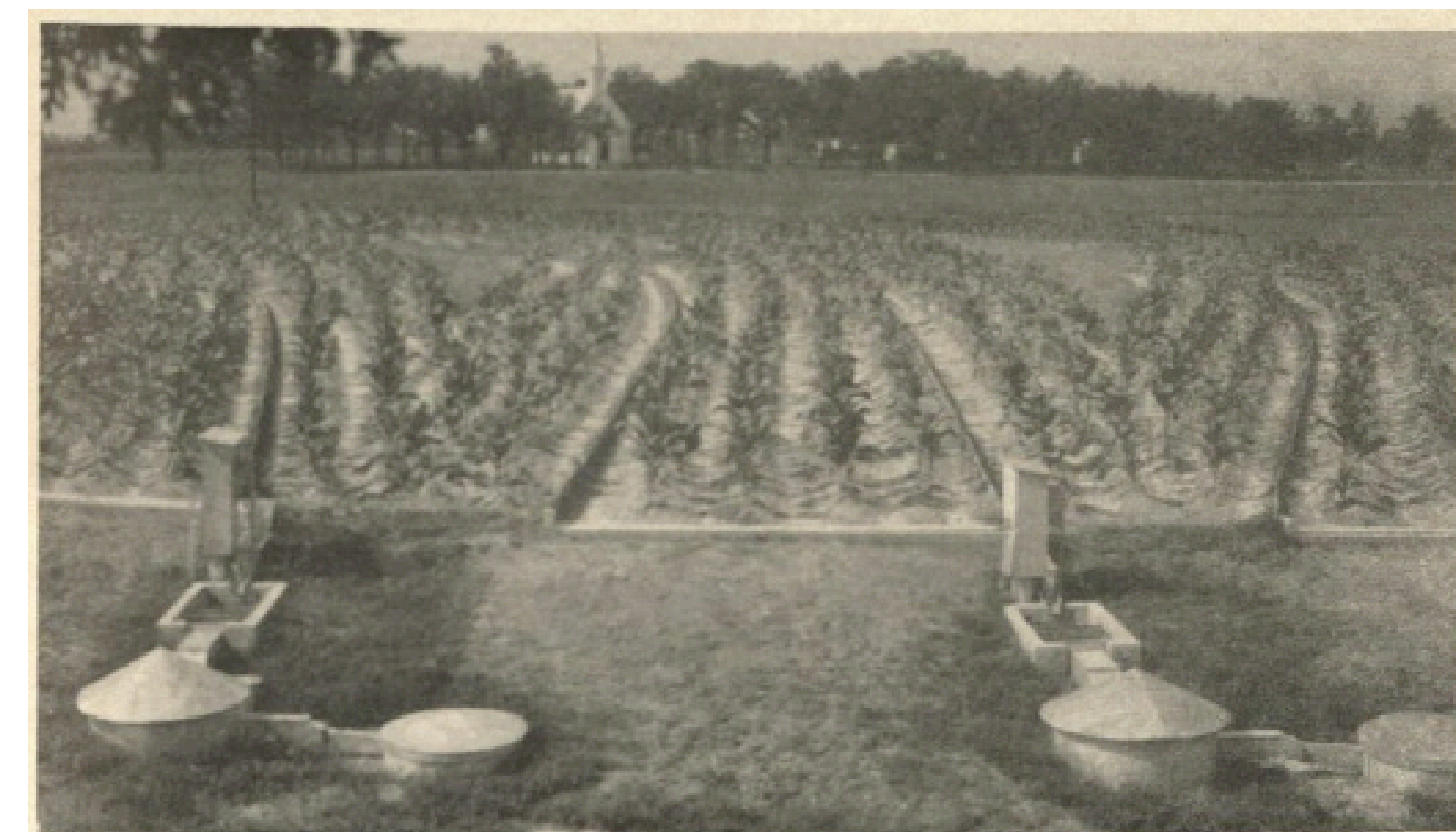
Figure 1. Runoff plots and catchment equipment from which soil and water loss measurements were made.
